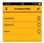
*Environment mode*: Indicate if your camera is installed inside or outside. In Europe you have to select 50 Hz.
