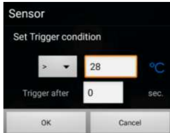
Figure 5-5: Temperature trigger condition.
