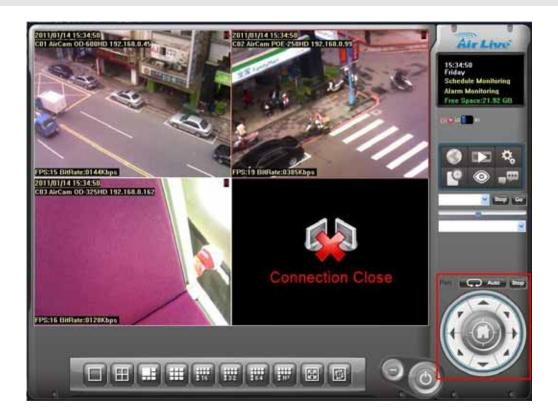
If the focused camera is with PTZ capability, the panel will show PTZ control button(s). A PTZ camera will enable all control buttons but a PT camera will enable PT control buttons only.
