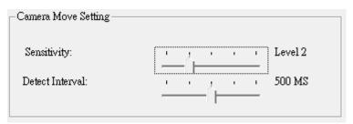
higher level to trigger camera move alarm easier, otherwise set lower level to prevent false alarm.
