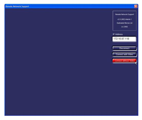
Enter the IP address of the Digital Multiplex Recorder you wish to configure, and click on 'Connect with Video' or 'Connect without Video'. The IP address may already be entered if you are accessing the network setup function using the Network Viewing software.
