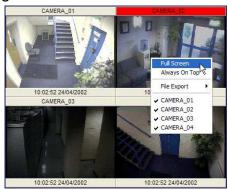
Cameras can also be displayed in a maximised view by right clicking the image and selecting 'Full screen'. The image can be returned to normal view by rightclicking the image again and selecting 'Restore'. If the aspect ratio is incorrect when viewing in a full screen, select the 'Aspect ratio' option to re-size the image.
