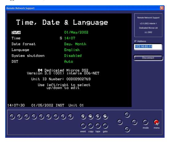
The menus you see are identical to the menus that are configured at the unit locally, and operation is the same at being at the unit. Click on the cursor keys to move the highlighted cursor around the screen, and edit the options. Click on the 'menu' button to move to the next menu page.
