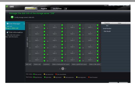
Select a disk in the disk table, the relative properties of the disk will be shown on the right, such as "Slot", "Serial Number" and "Disk Model".
