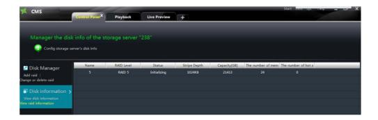
Click Add raid button, you can add new raid. Input the raid name, select raid level and stripe depth, click button to add raid.
