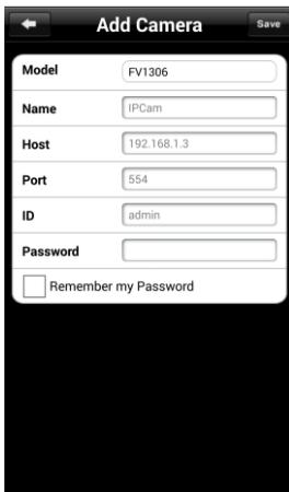
4. After entering all necessary data, select **Save** to save the camera to Camera List.
